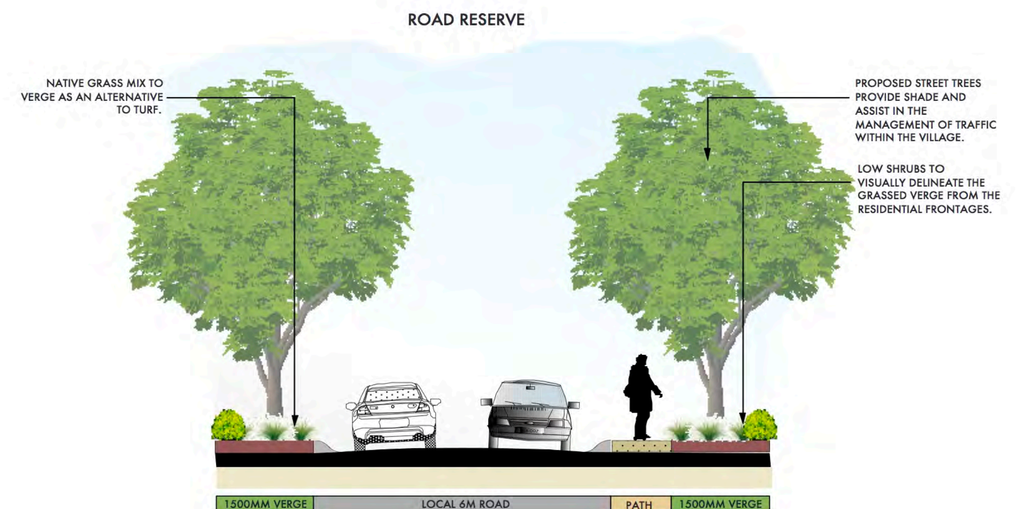
S04 TYPICAL INTERNAL ROAD TREATMENT LP06 Scale: 1:75
